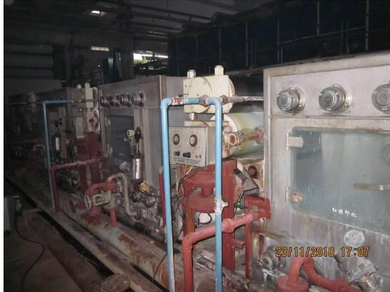
Picture 2: Wash Boxes after Mercerization at Kamal Limited
